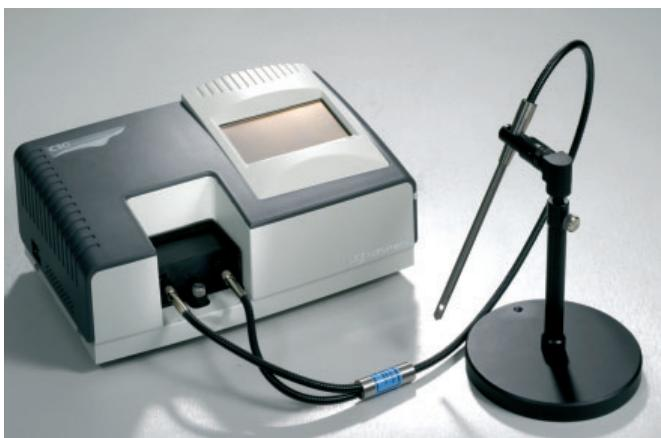
Use the fibre dip probe for in-situ sample measurements.
