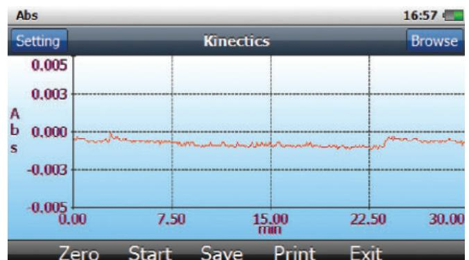
The Kinetic workspace enables the measurement of Absorbance or Transmission as a function of time. Use the zoom and peak pick features to obtain a better view of the Kinetic curve. Measurement data can be saved and recalled at any time.
