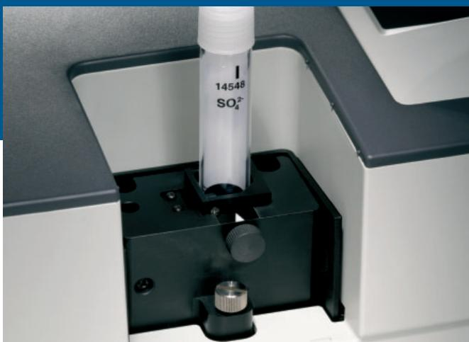
Use the universal cell holder to measure various pathlength rectangular cells and rounds test tubes accommodating all of your sampling requirements.
